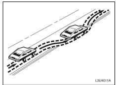
If the level of the shoulder is only slightly below the pavement, recovery should be fairly easy. Ease off the accelerator and then, if there is nothing in the way, steer so that your vehicle straddles the edge of the pavement. You can turn the steering wheel up to one-quarter turn until the right front tire contacts the pavement edge. Then turn your steering wheel to go straight down the roadway.
